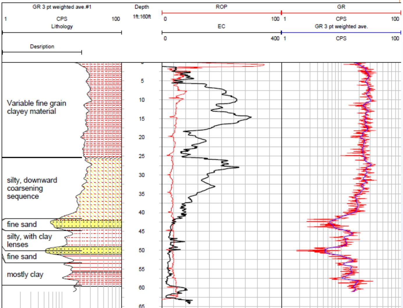
Fig.1 An example data set/Gamma Log derived from data obtained using the nano gamma probe. Courtesy of Mount Sopris
