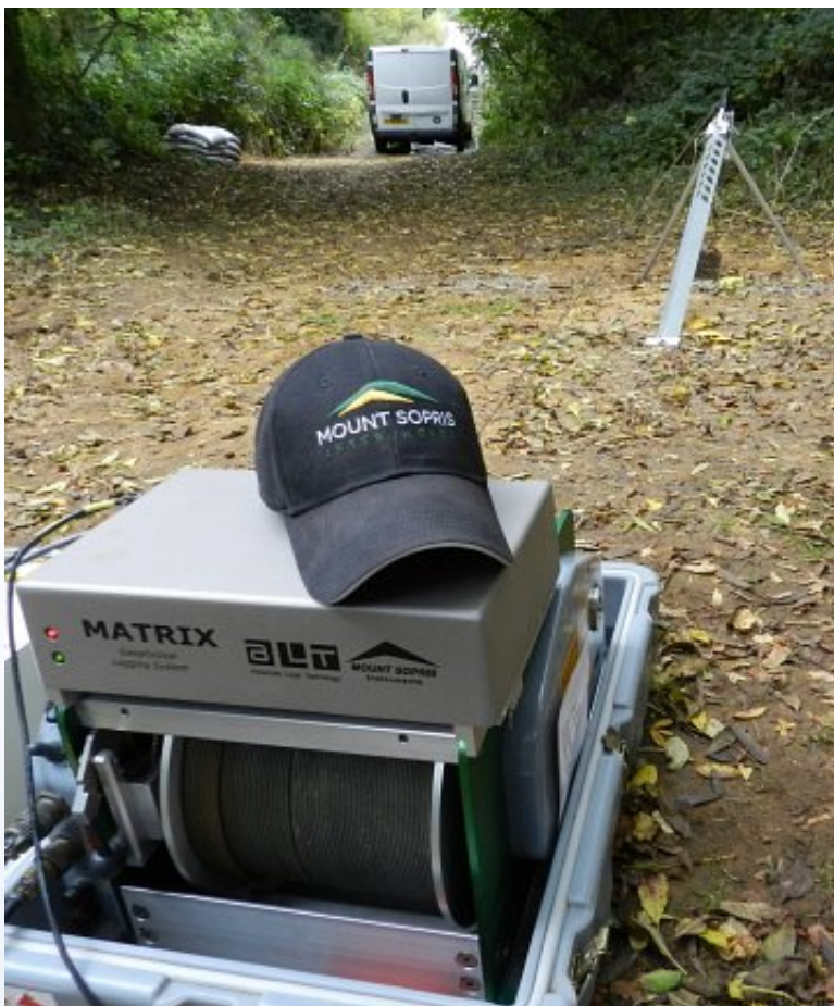
Matrix Logger installed onto MX Winch.
