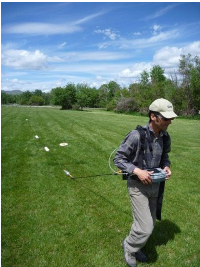
OhmMapper in operation with Geometrics console (Courtesy of Geolex Inc., Helena, Montana USA)
