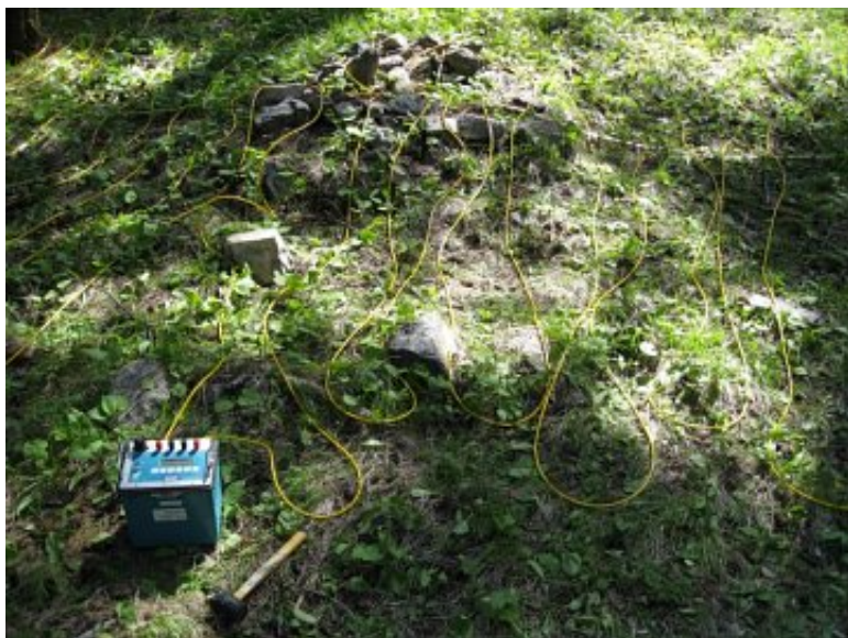
Syscal Kid in operation by student at the University of Montana (Image Courtesy of the Department of Geosciences, University of Montana, USA).
