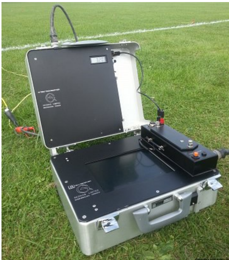
The bottom of the case holds the recording electronics and data acquisition interface, whilst the lid contains a TEM47 transmitter.
