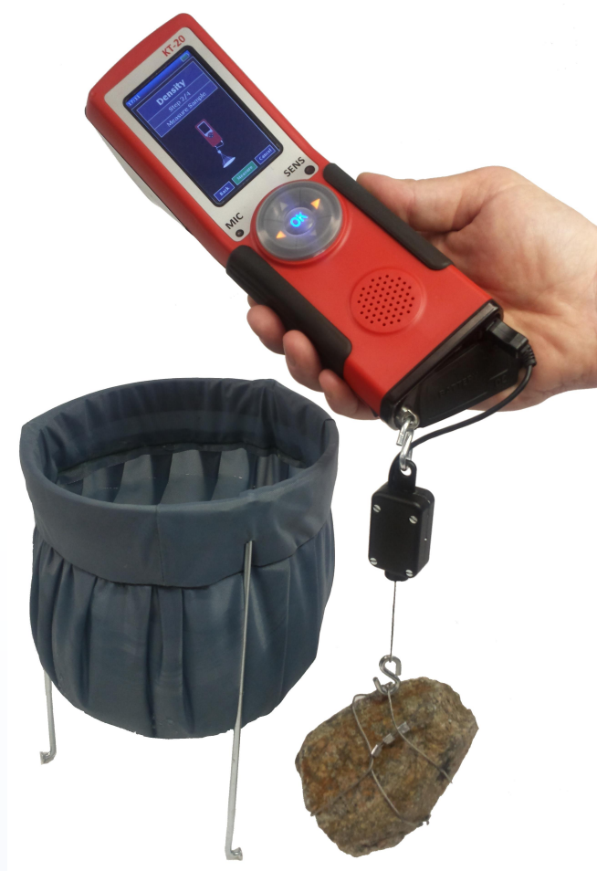
KT20 density measurement- first the sample is weighed in air. Image courtesy of Terraplus..
