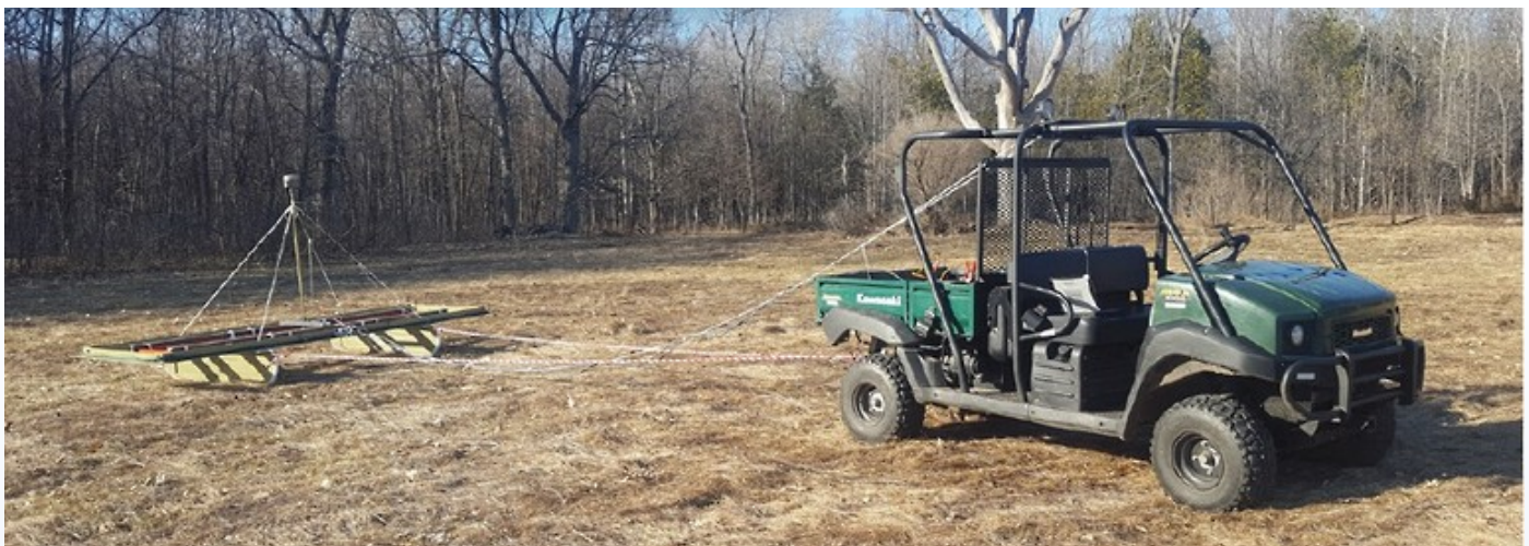
Fig.1. Showing the typical survey set up and tow vehicle arrangement of the EM63 Flex (Image courteously provided by Geonics)
