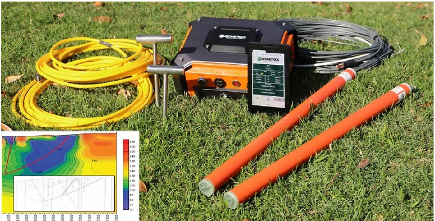
Fig. 1. Shows the Stratagem EH-5 components which includes the Stratagem console, Android tablet, stakes, cables and mag coils. The image on the left is a 2D inverted dataset from a mineral exploration study using the EH-5 showing a 65°-75° striking fault, close correlation to the geological map of the area (Image Courteously provided by Geometrics Inc)
