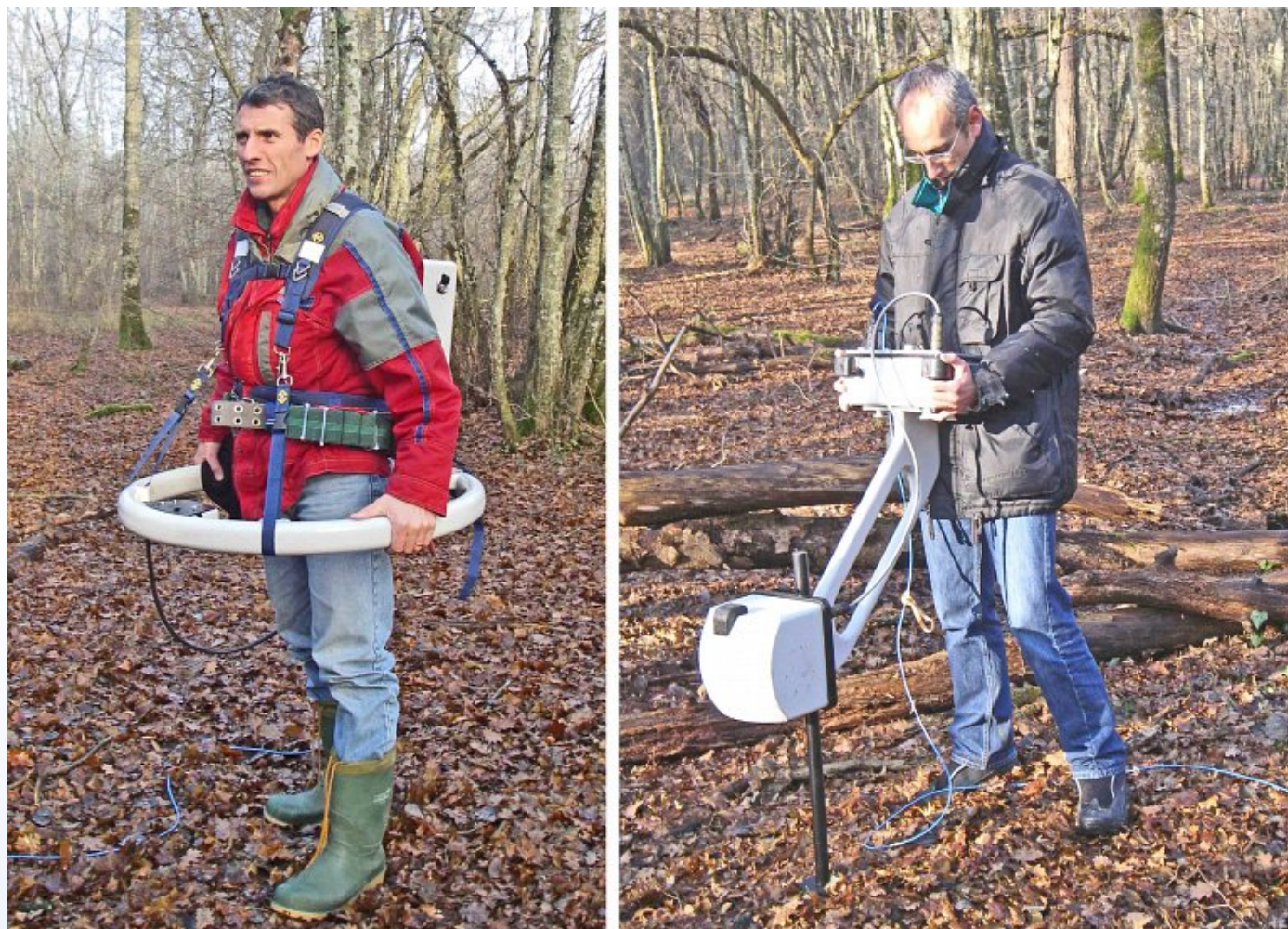
The PROMIS Transmitter coil (left) and 3 component receiver (right) in operation. Image courtesy of Iris Instruments.
