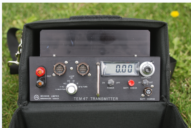
TEM47HP, note the attentional heatsink. Image courtesy of Geonics Limited.
