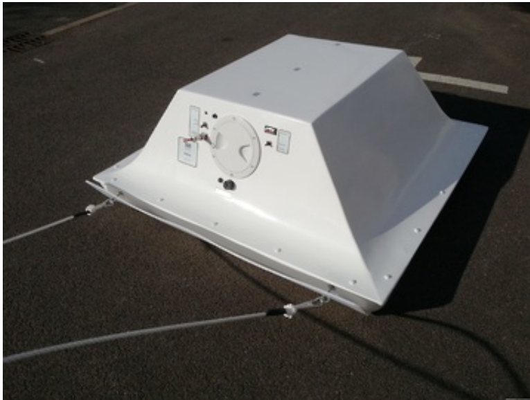
GroundVue 100 with trailing odometer wheel.
