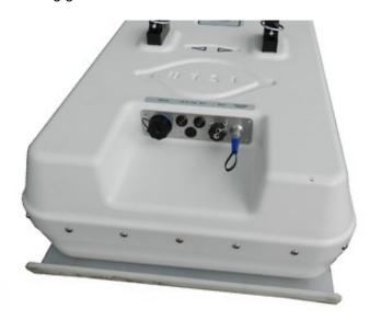
Weighing less than 7kg the system is light and portable for deploying in remote difficult to access locations. An internal GPS chip time stamps each record and can be used for data quality control – for instance confirming the heading of each traverse. An external GPS, RTK GPS or total station can be integrated with the radar data for precise geospatial positioning.
