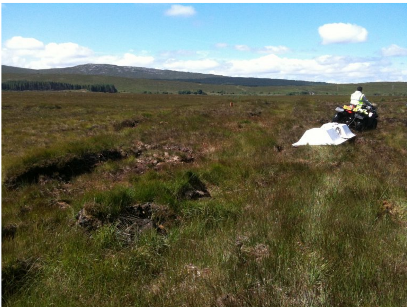
Picture of the GroundVue 2 being used to assess the depth of peat. Image & video courteous of Atlas Geophysical Ltd.
