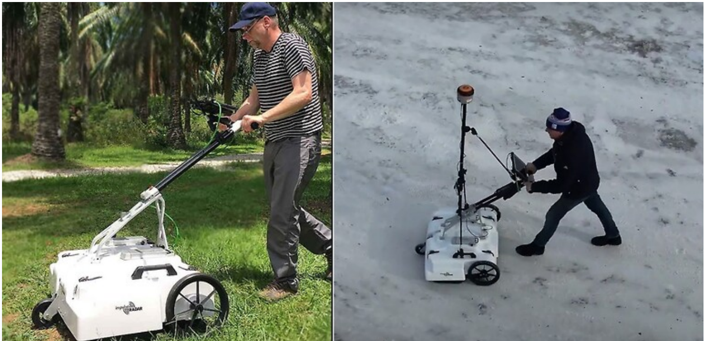
Fig 1. Image showing the typical arrangement of the Cart Raptor GPR series in different environments.
