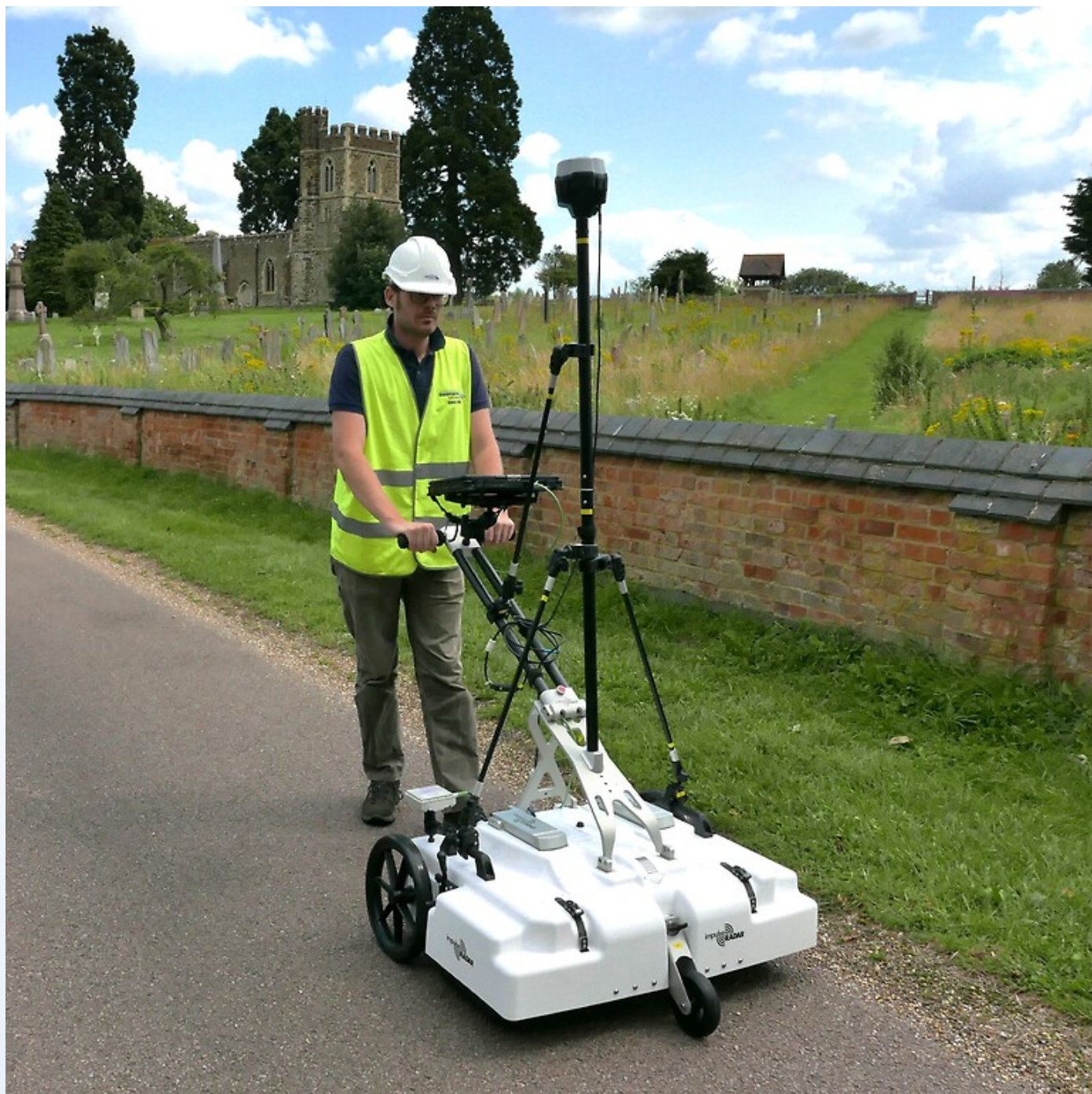
Fig 1. Image showing Raptor cart system being used for utility detection.
