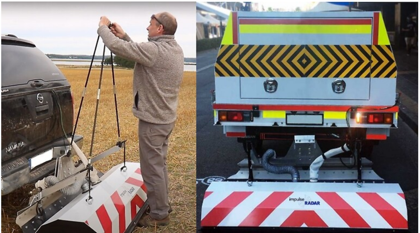
Fig 1. Shows the features of the vehicle carrier and how it fixes onto a survey vehicle
