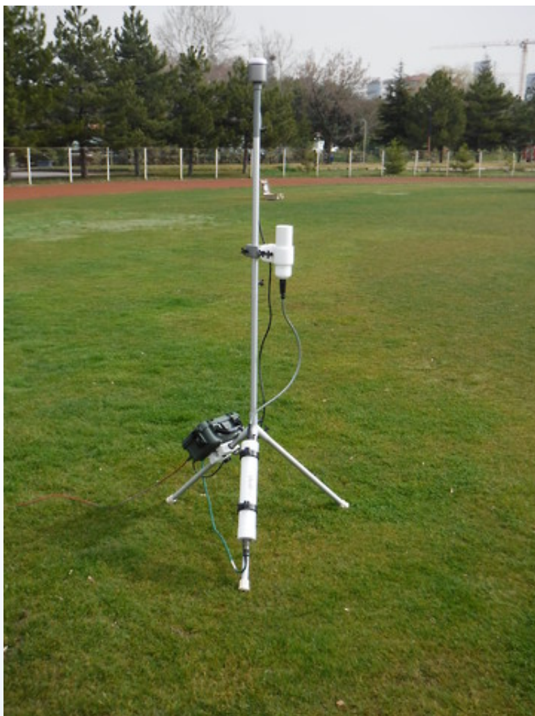
G-862 magnetometer basestation configuration with GPS and data recording module. Image courtesy of Geometrics Inc
