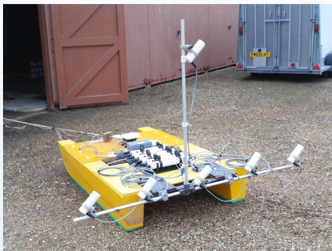
Magnetometer array installed on the Geomatrix MSP Sledge. Image courtesy of English Heritage.
