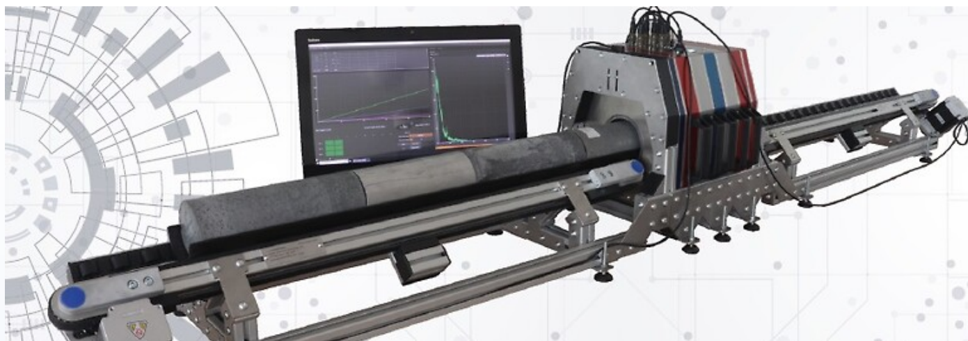
Fig. 1 Full length image of the gamma ray core sampler comprised of the measurement section with 3 detectors and the conveyor system including a rock core sample which is being analysed (Image courteously provided by Georadis)
