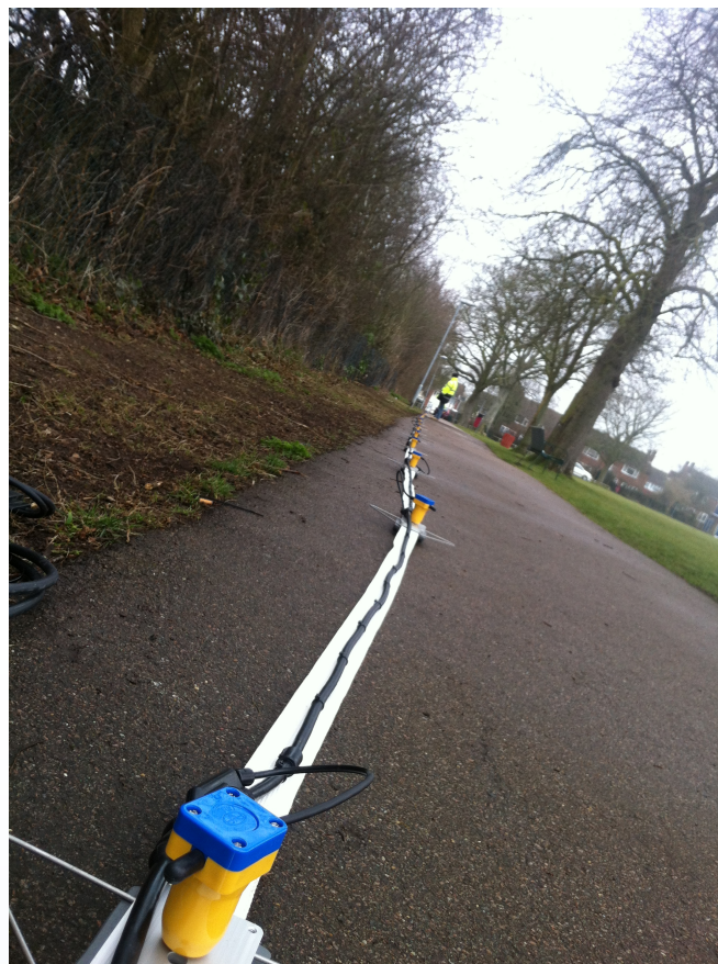
Here is an example of a 48 channel single component landstreamer.
