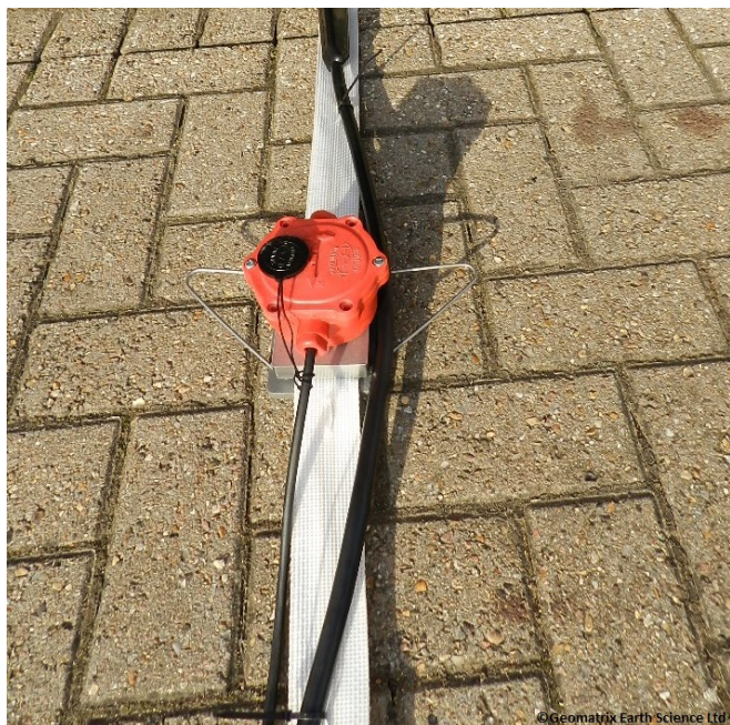
Landstreamers with 3 component geophones can be supplied with up to 48 channels.
