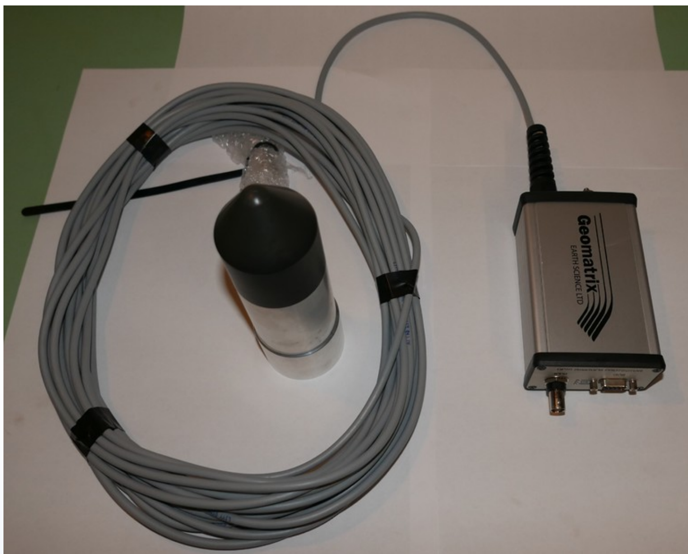
Fig.1. Image of the SmartGPS-3TP and the Geomatrix GP111 Smart GPS protector, connected via the 200m cable.
