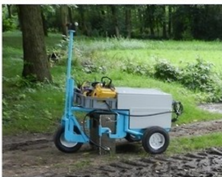
Lightning Seismic Vibrating source mounted to an ATV for deployment on difficult terrain.
