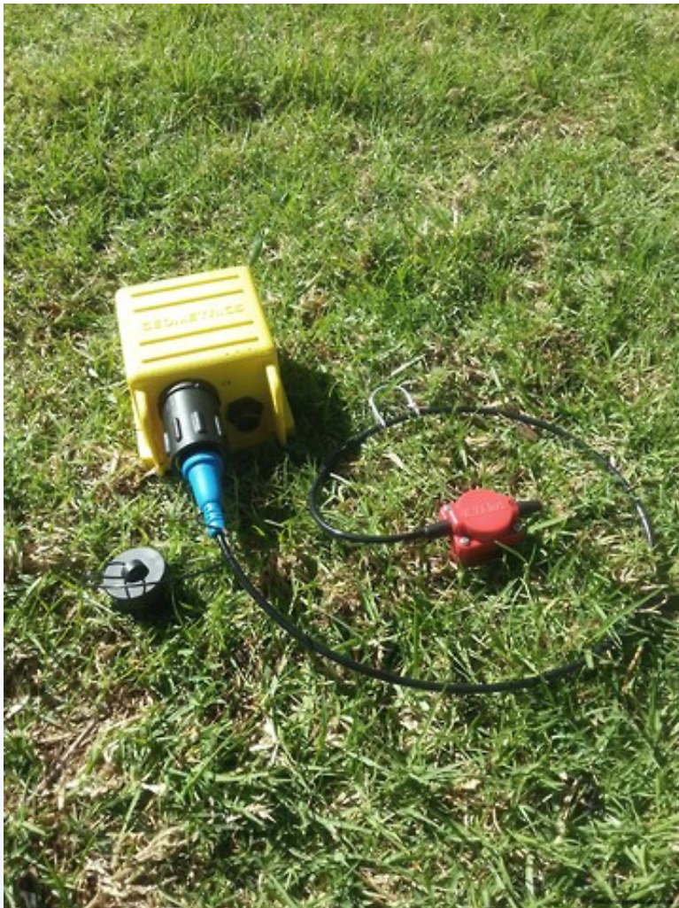
Atom Seismograph installed on station with 2Hz vertical Geophone.
