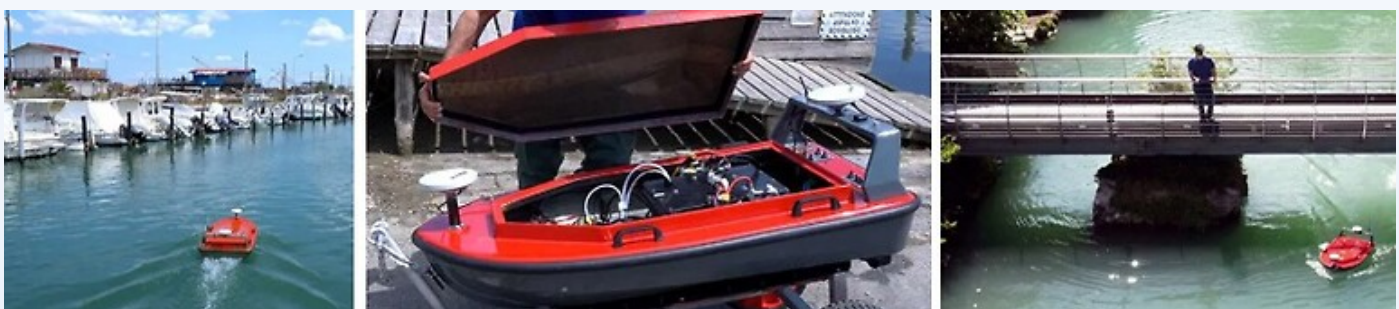
Fig 2. CK-14 Surface autonomous vessel in use within a harbor and wide river (shallow water environments) as well as an image of the internal electronics, power and housing in which you can connect any serial devices. Image courteously provided by Codevintec Srl.
