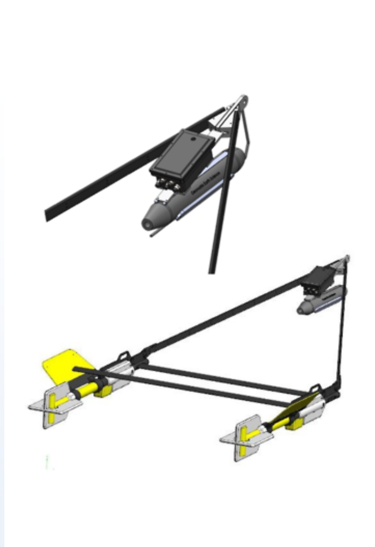
Drawing illustrating the deployment of the QAS? telemetry system on a Transverse Gradiometer Frame with integrated Side Scan Sonar.
