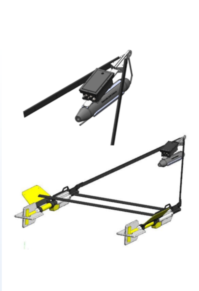
Drawing illustrating the deployment of the QAS4 telemetry system on a Transverse Gradiometer Frame with integrated Side Scan Sonar.
