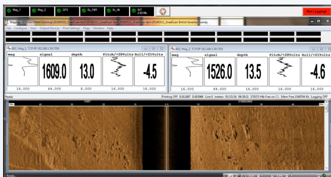
QAS4 SideScan Sonar Image of a Ship Wreck
