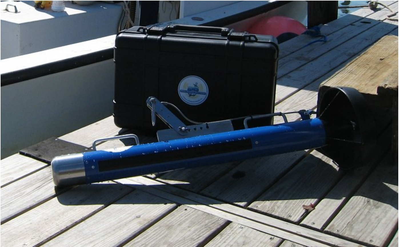
HMS-1400 Side Scan Sonar ready for deployment. Image courtesy of Falmouth Scientific Inc.
