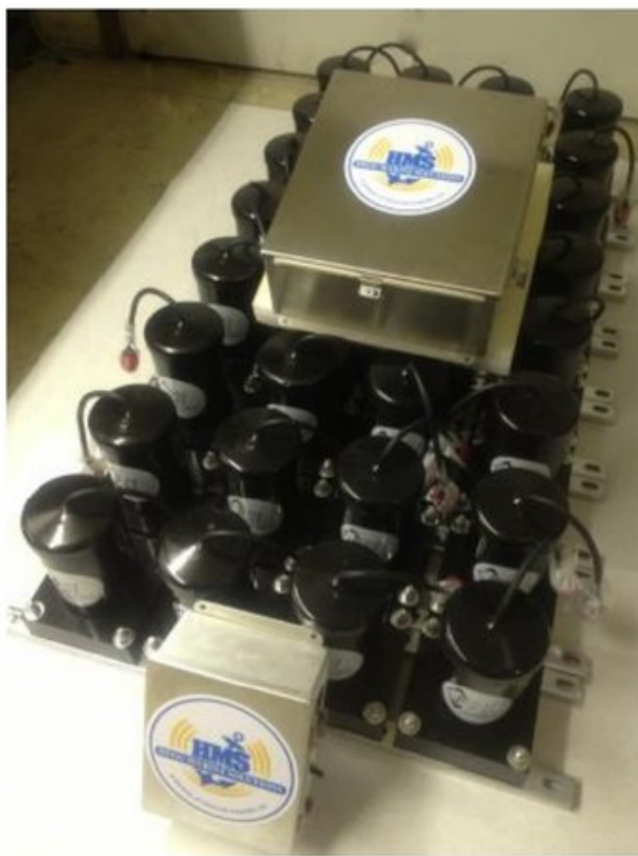
Fig.2. Image of a typical low frequency array with J-Boxes (Image courteously supplied by Falmouth Scientific)
