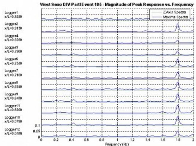
*Example Vortex Induced Vibration (VIV) and Drilling Induced Vibrations (DIV) events. Courtesy of Falmouth Scientific Inc.*
