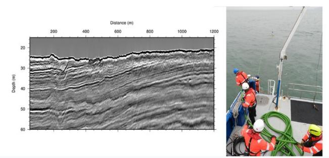
In addition to the higher 16kHz sample rate the GeoEel LH-16 also boast a much higher data transfer rate to allow for up to quarter second shot intervals (with a 48 channel array) with sparker and boomer sources.
