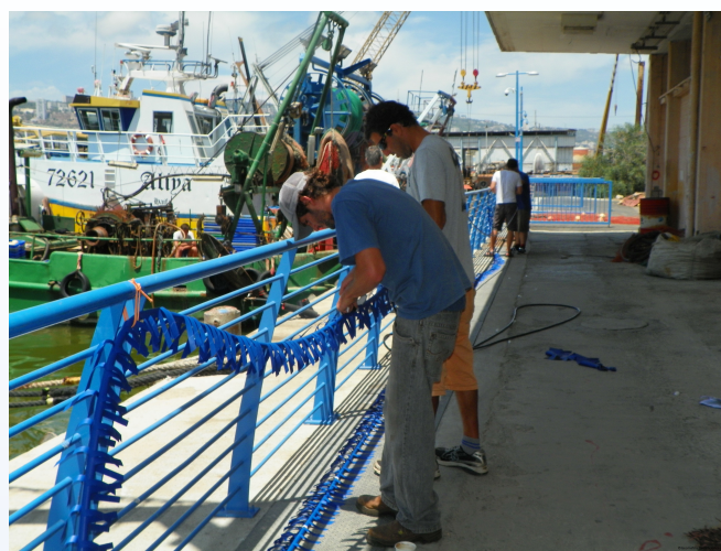
Adding fairing to GeoEel tow cable to reduce noise on the streamer due to cable strumming.
