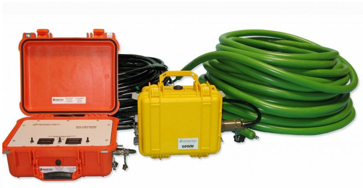
MicroEel System with Geode Seismograph. Image courtesy of Geometrics Inc.
