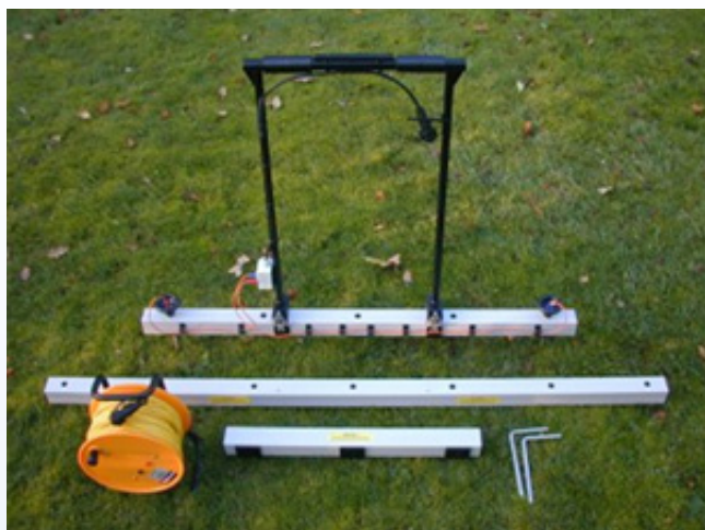
PA20 Frame with 0.5m, 1m and 1.5m beam, plus remote electrodes and remote cable.
