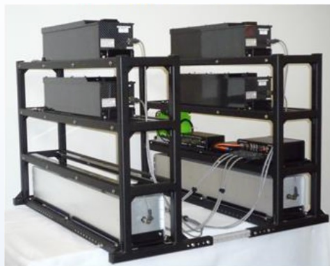
RS700 system with 4 x 4 RSX-1 gamma spectrometers and RSN-4 Neutron detector. This detector configuration permits lateral target discrimination. Image courtesy of Radiation Solutions Inc .
