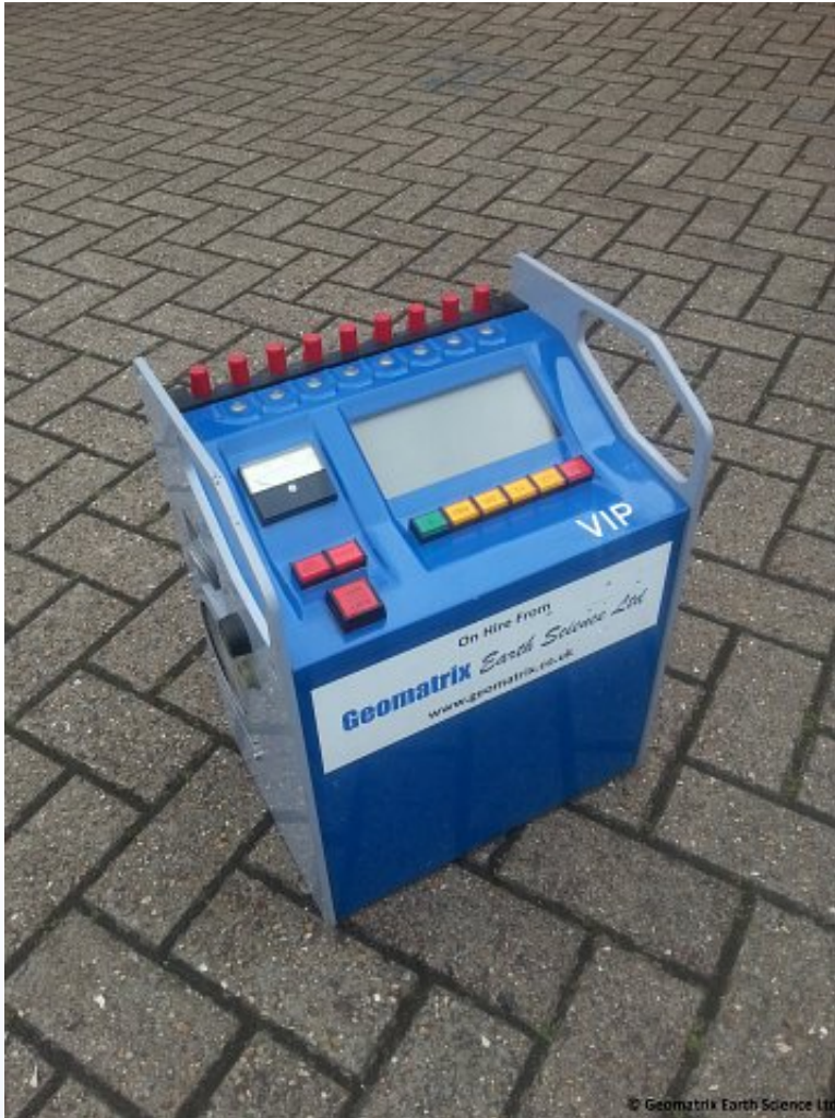
VIP 3000 Resistivity and IP transmitter.
